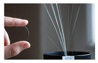
temperature, pressure, stress, torsion, or position of your material with a tool thinner than a grain of sand. It is affordable and also quick and easy to manufacture as per specific requirements. Passive measuring is based on micro-wire technology and magnetic fields with no need for power sources. The elastic, anti-corrosive, and undestroyable sensor can be placed in any material without affecting its properties or environment.
